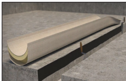
Apply the VEDACOLLE ® adhesive to the inside edges of the joint on a depth of 90mm.
