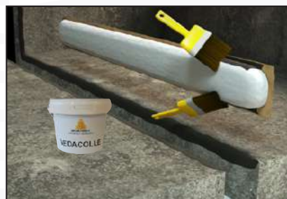
Apply the VEDACOLLE® adhesive under the wings and on the vertical side of the blanket on a width of 6cm.
